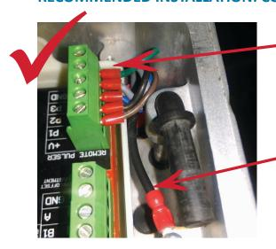
Cores terminated with bootstrap ferrules (8mm pin length x 1.5mm ø).
